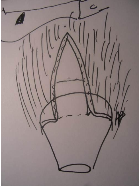
Figure 10 : V shape Tear
